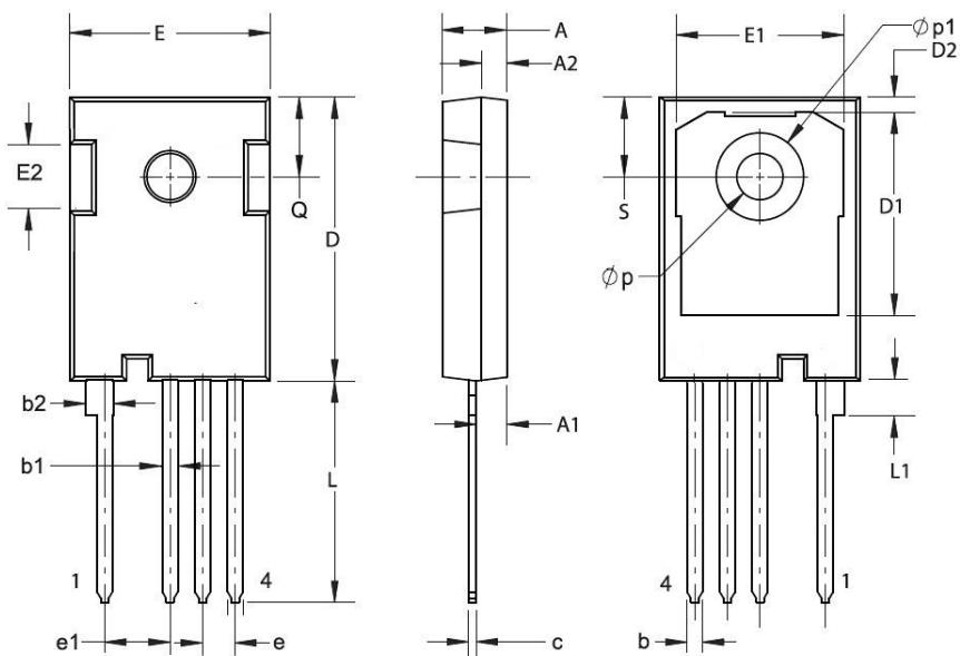
Note: 1:Drain(D), 2:Source(S2), 3:Source(S1), 4:Gate(G)
