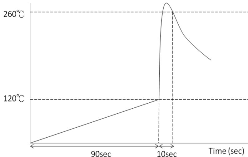
Solder capacitors under the soldering conditions as follows.
